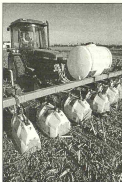
Hooded sprayer units direct herbicides directly between the rows of crops greatly minimizing drift.
