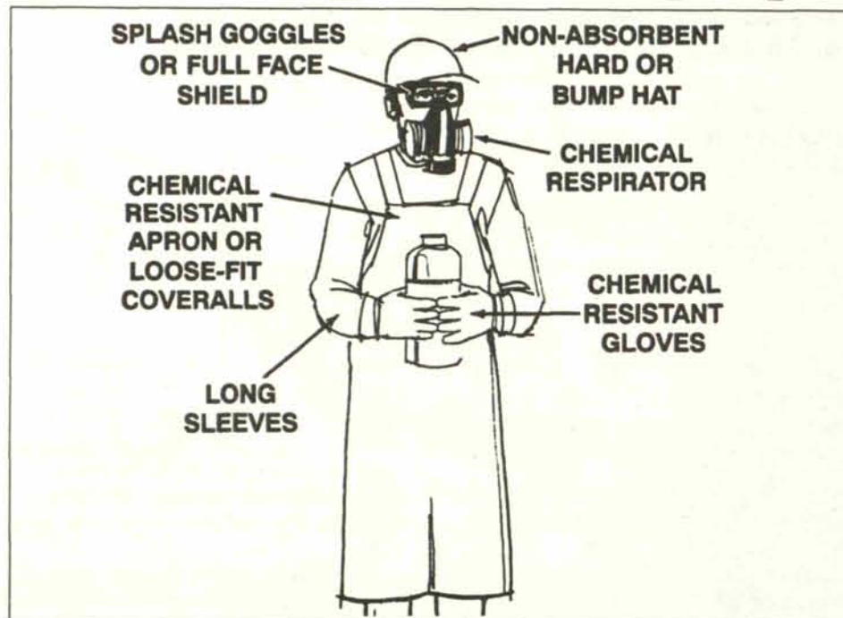
Use personal protective equipment when working with pesticides, such as what is recommended above.
