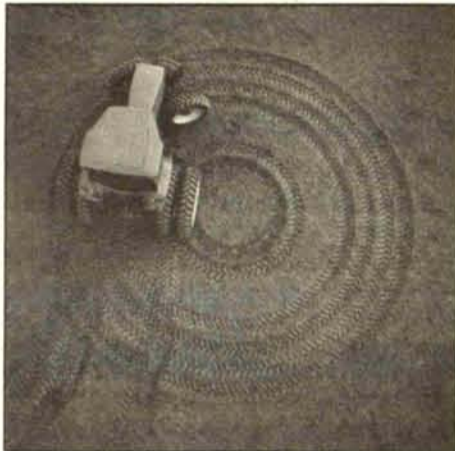
SuperSteer FWD allows the tractor to turn on a dime...15-feet exactly, with any size tire.
