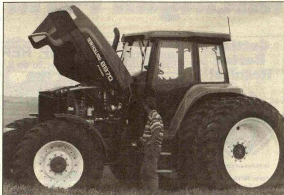
Genesis' hood lifts like a car's to expose the engine, allowing for no-hassle maintenance.
