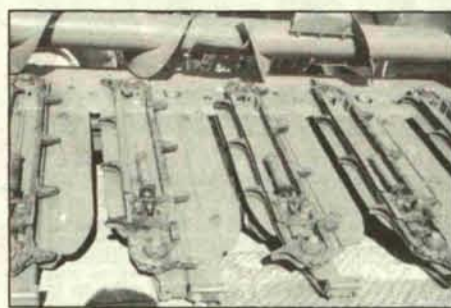
The first of its kind, produced by Rod Van Middlesworth, this 16-row John Deere narrow row corn head was originally an eight-row head. Van Middlesworth had to extend the sides of the head by 6 inches to accommodate the eight extra rows. He estimates it cost him $2,000 per extra row installed on the corn head.
