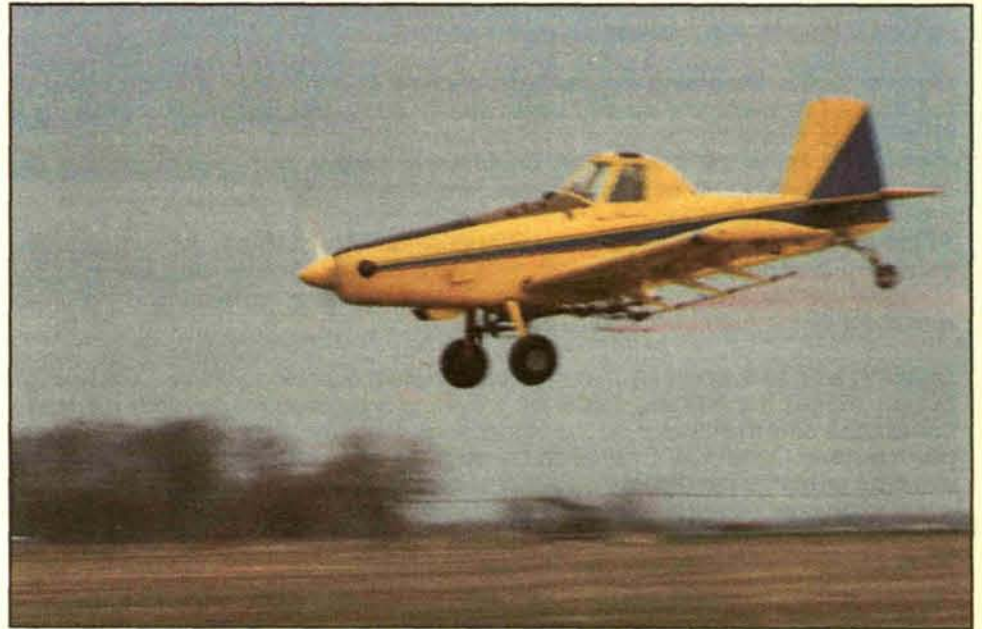
Traveling at 140 miles per hour, just three to five feet off the ground, this Air Tractor AT-400, manufactured in Texas, makes a pass across the string and test cards during the calibration trials at the fly-in. The plane, flown by Mike Schiffer of A1's Aerial Spraying from Ovid, is powered by a 680-horse Pratt and Whitney turbo-prop and is equipped with a 400-gallon hopper.
