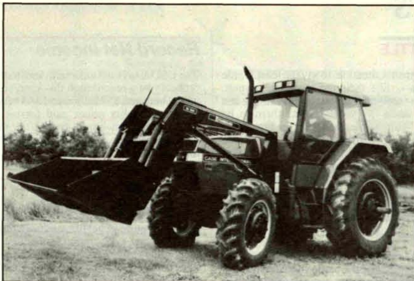
NEW FROM FARMHAND: Farmhand's Model XL740 and XL940 loaders now mount both two wheel drive and front wheel assist Maxxum 5120, 5130 and 5140 tractors; the model 22 loader mounts the two-wheel Maxxum tractors. Loader features include Farmhand's exclusive Quick-Tach for fast tractor hook-up and parking stands. Typical lift height on the XL940 loader is 12'8", XL740 is 10'6" and model 22 is 10'4". Options include heavy duty buckets, manure fork, grapple fork, and large round bale spear. For more information, contact Farmhand, Inc., P.O. Box 1500, Excelsior, MN 55331 or call (515) 236-6571.
