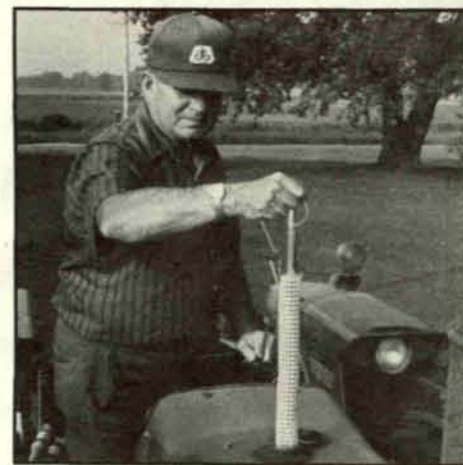
Water Dog absorbs up to 400 times its own weight in water to help prevent fuel contamination, clogged filters, fuel line freeze-ups, and tank rust. According to the manufacturer, Water Dog is available in sizes to fit farm tractors, combines, trucks, small engines, and farm fuel storage tanks. For more information, contact AGA National Products Group at 1-800 876-9423.
