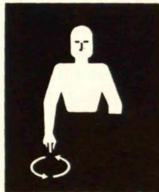
FIG. 10—LOWER EQUIPMENT—Make circular motion with either hand pointing to the ground.
