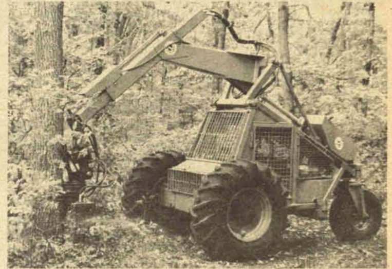
A new type of logging equipment being used to harvest timber in the Oak Haven forest is the Mor-Bell Logger. Designed in South Africa by Irvin Bell and manufactured by Morbark Industries of Winn, Mich., the Logger is able to thin woodlots without damaging other trees. The Logger is front equipped with a hydraulic shear which "snaps" the tree, leaving no debris around the truck, as shown in the photo below. After snapping the tree, the Logger is able to "carry" the felled tree and place it with others for removal from the woodlot.
