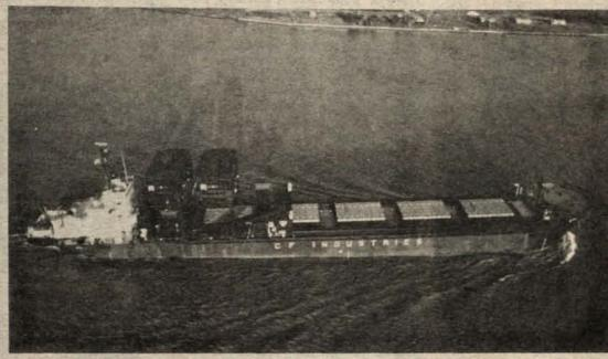
CF Industries integrated tug-barge was christened recently at Port of Tampa, Florida. This innovation in water transportation comprises independent tug and barge components that are joined during service and may be detached during cargo transfer. Ownership of the "Jamie A. Baxter" includes Farm Bureau Services, Inc. and 18 other North American farm supply cooperatives.
