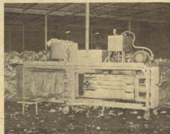
SPACE-SAVER — is this new, heavy-duty wool baler which compresses the fleece into storable 500-pound bales.
