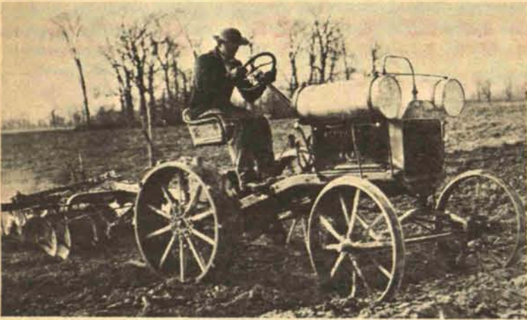
THIS EXPERIMENTAL TRACTOR — was one of more than 50 produced by Henry Ford in search for cheap farm mechanical horsepower. In this version, Model T gas and water tanks were mounted above the engine. The Ford company will soon observe the 50th anniversary of the world's first mass-produced tractor.
