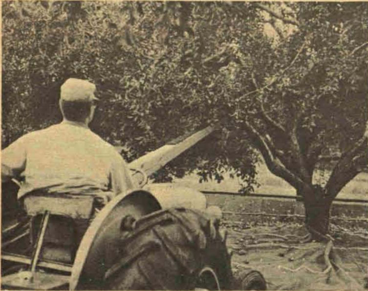
APPLE SHAKER—is shown in operation at the Herbert Teichman orchard near Eau Claire, Michigan. Through mechanization, Michigan growers are attempting to overcome the drastic labor shortage. Teichman was first to mechanically harvest Michigan apples for processing on a commercial scale.
