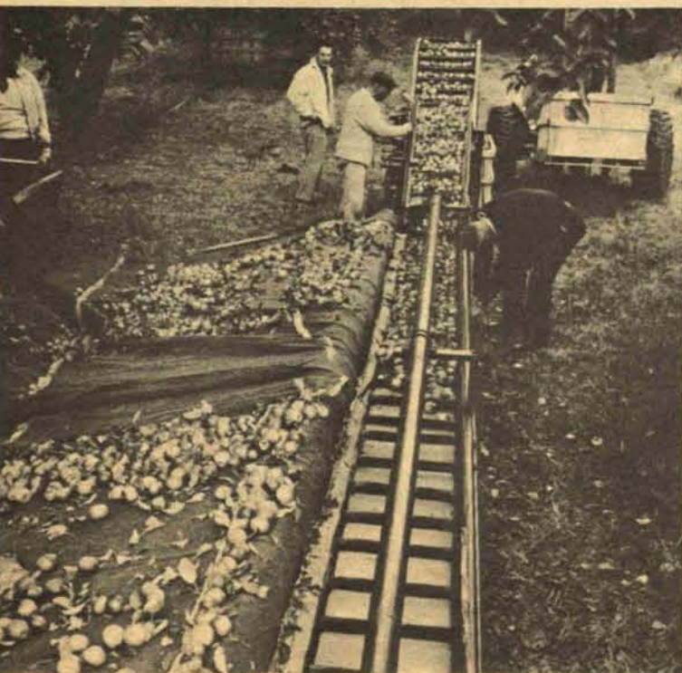
MECHANICAL MOVING—of the fallen apples to the conveyor is handled hydraulically by a "rewinding sheet". Some loaders include blowers to remove leaves and trash. Many growers used mechanical harvesting this year on an experimental basis and most agree that practical systems will soon appear.
