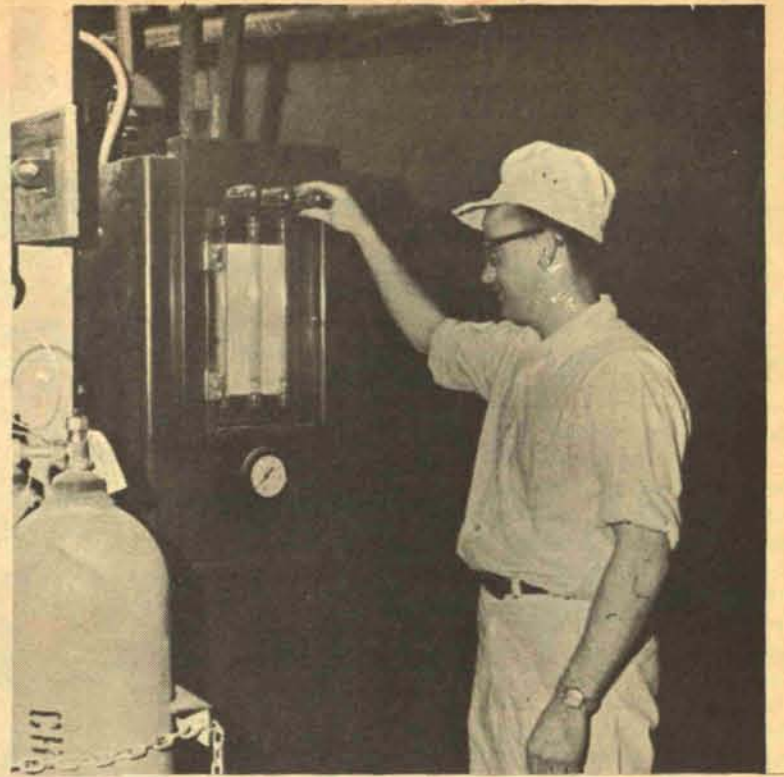
BLEACHING FLOUR — from its natural creamy color to a pure white product is performed in an agitator through which flows a deadly gas — chlorine. The gas is carefully metered from the bottles to the bleaching unit.
