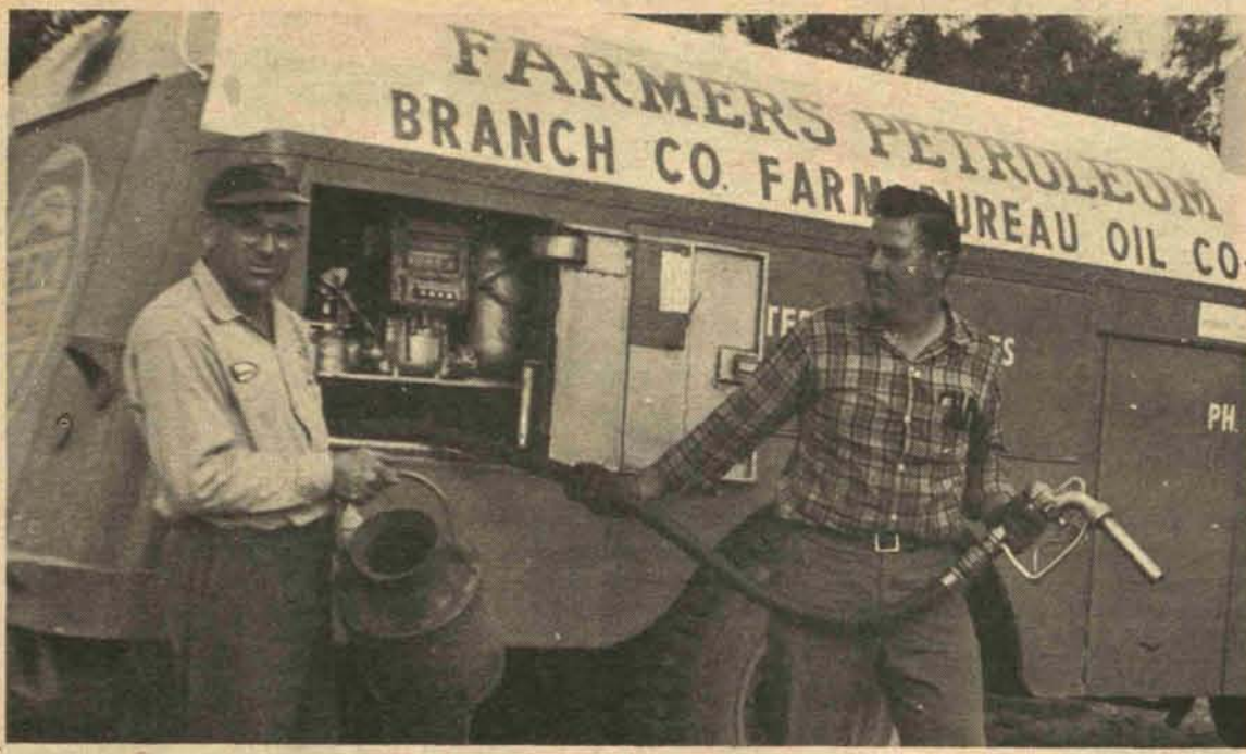
THE MODERN PETROLEUM "TANKER" —with its electric pumps, meters and many yards of hose— means quick, efficient delivery of fuels. Manager Clarence King shows driver Bob AcMoody the old 5-gallon measuring bucket that did the job when the cooperative began filling farmers' tanks in the '30's.
