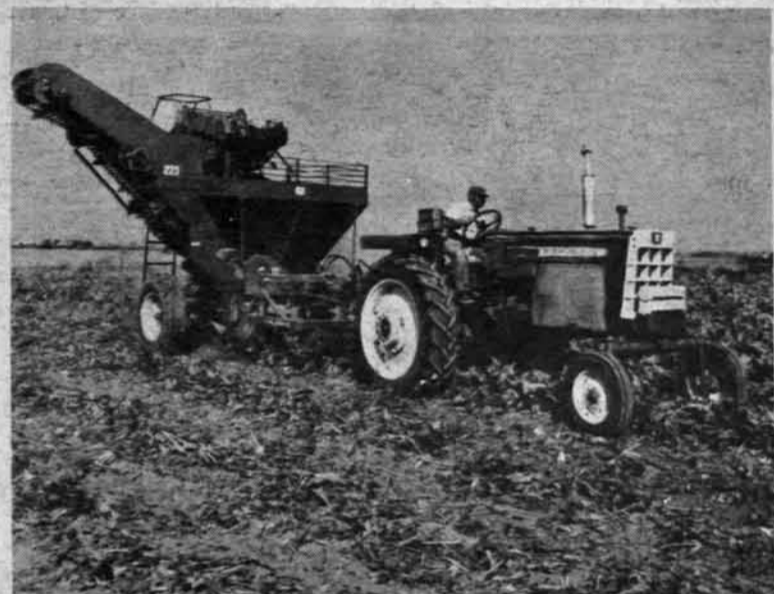
THE SUGAR BEET HARVEST, once a back breaking laborious job, is 100 percent mechanized today. Michigan farmers using the latest mechanical harvesters are able to harvest from 10 to 15 acres of beets during a single working day.
