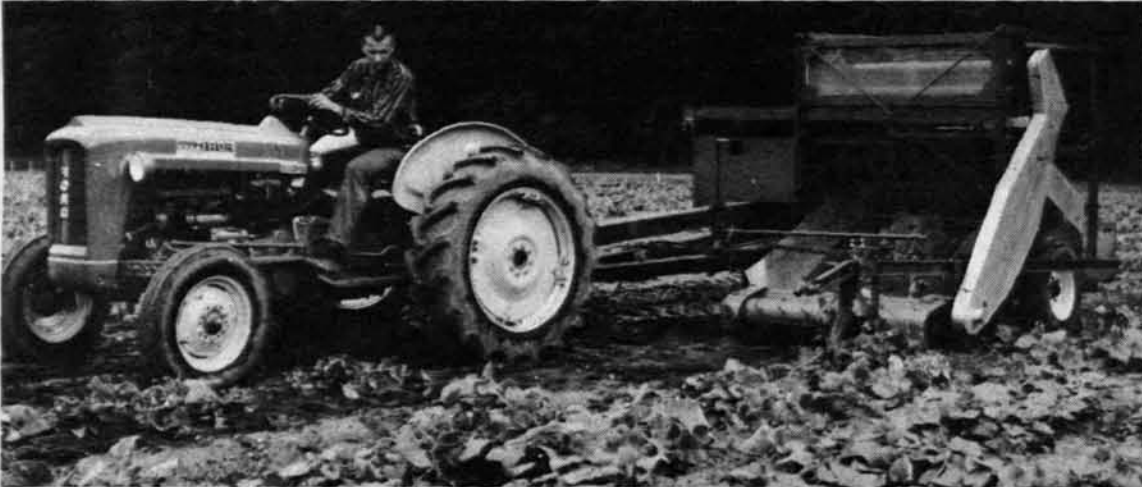
NEW MSU CUCUMBER HARVESTER is a once-over machine that operates by lifting the plants from the soil and running them between a pair of rubber belts. The fruits are stripped from the vine and fall into a conveyor which places them in any suitable container. Although the machine is the result of three years of research, it will be several more years before commercial production can be achieved.
