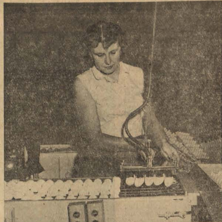
PNEUMATIC LIFTER—removes eggs from shipping cases onto the flash candling table at the Jenison egg-processing plant of Farm Bureau Services. Similar modern devices will be installed in the proposed second unit scheduled to be built.
