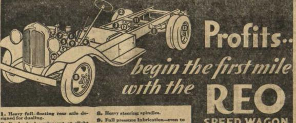
2. Dual wheel equipment at slight 3. Heavy 7' channeled frame. 4. 4-speeds forward transmission 5. Big truck engines-4 or 6 cylinder.
