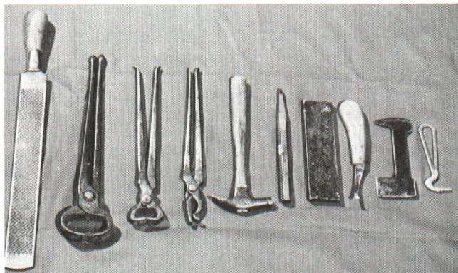
Figure 1. Farrier tools include, L-R, rasp, pincher, hoof nipper, nail clincher, hammer, punch, clinch bar, knife, clinch cutter, and hoof pick.
