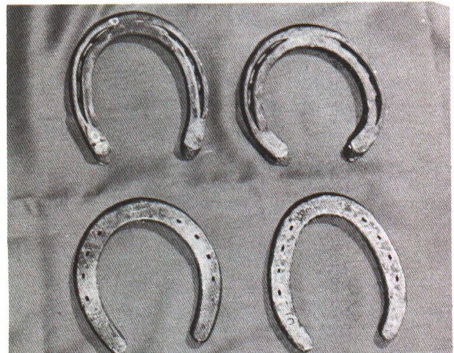
Figure 6. Top are unfitted and fitted front shoes. One on right has been rounded by spreading the toe and turning in the heels to fit a pattern. The lower right shoe has been narrowed at the toe, spread at the branches, and turned in at the heels to fit a hind foot. Its mate has not been shaped.
