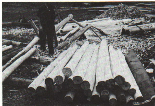
If cedar is to be treated or finished, all the bark must be removed as is being done here.
