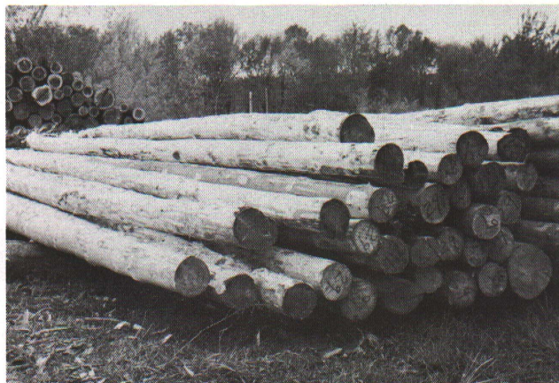
Cedar poles debarked and awaiting use. Maximum advantage is taken of cedar's decay resistance for this use.
