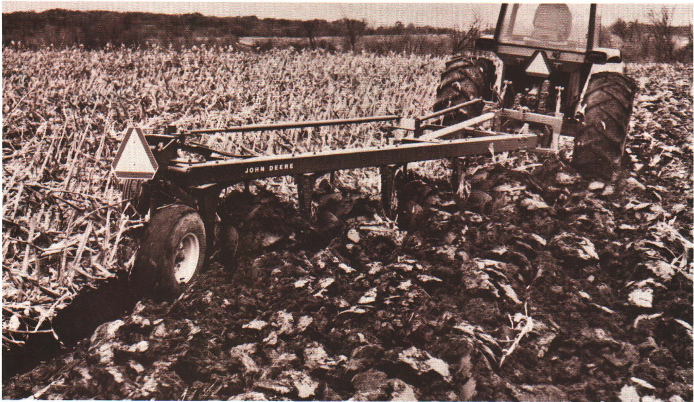
Figure 2. Early planted crops respond especially well to tile drainage. This compact soil contains more water than desirable. Tractor and plow wheels are in the furrow, deeply compacting the soil, thus slowing movement of gravitational water to the tile.
