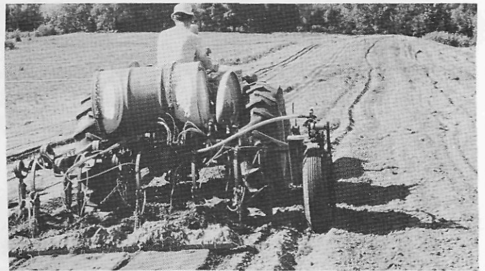
Figure 3. — A typical chisel type fumigant injector for use in pre-plant soil fumigation.
