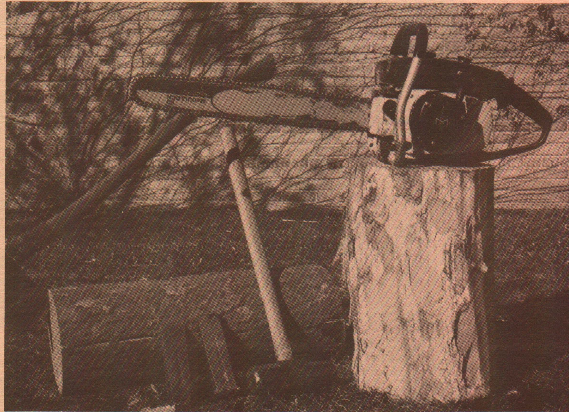
Figure 3. A minimum of tools is required to harvest your own wood. A chain saw makes for faster cutting, however a crosscut or bow saw may also be used. All of these tools can be obtained from local hardware or farm supply stores.
