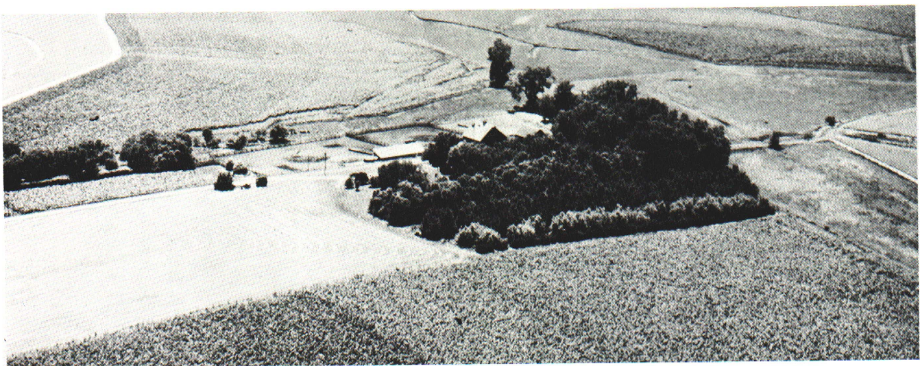
Figure 17. Trees can be very effective in reducing wind velocities when planted according to recommendations. Properly designed windbreaks modify wind speed and direction on the leeward side for a distance equal to approximately 40 times the height of the trees.
