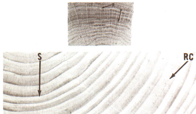
Figure 5—(Top) cross section of red oak, a hardwood with large pores, P; rays, R. (Bottom) southern pine, a softwood with dense latewood, S, and resin canals, RC (dark or light "spots.")
