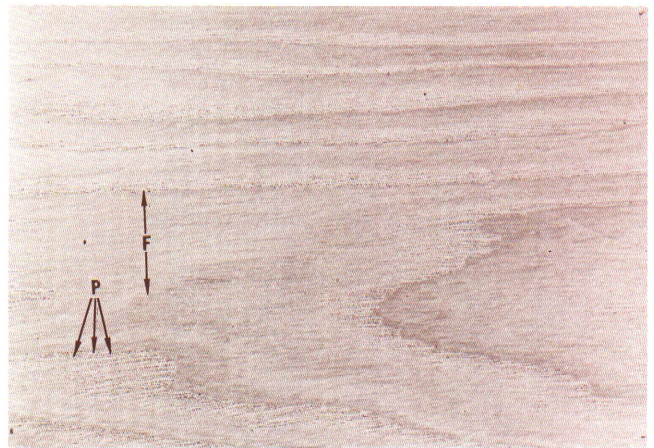
Figure 16—White Ash. Earlywood pores, P, poreless smooth areas, F.
