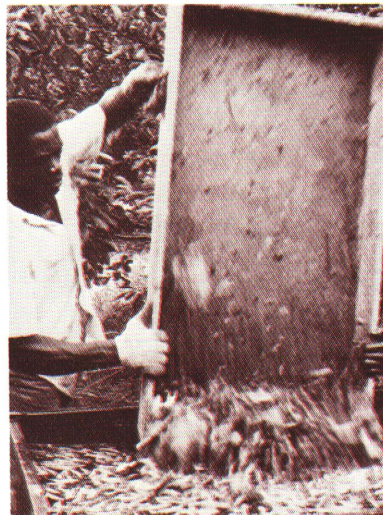
Fig. 7—An overloaded conveyor caused by an excessive harvesting rate. Overloading increases fruit damage, such as bruising and eventual scald.
