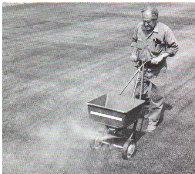
Centrifugal type fertilizer spreaders distribute materials rapidly with minimal overlapping problems.
