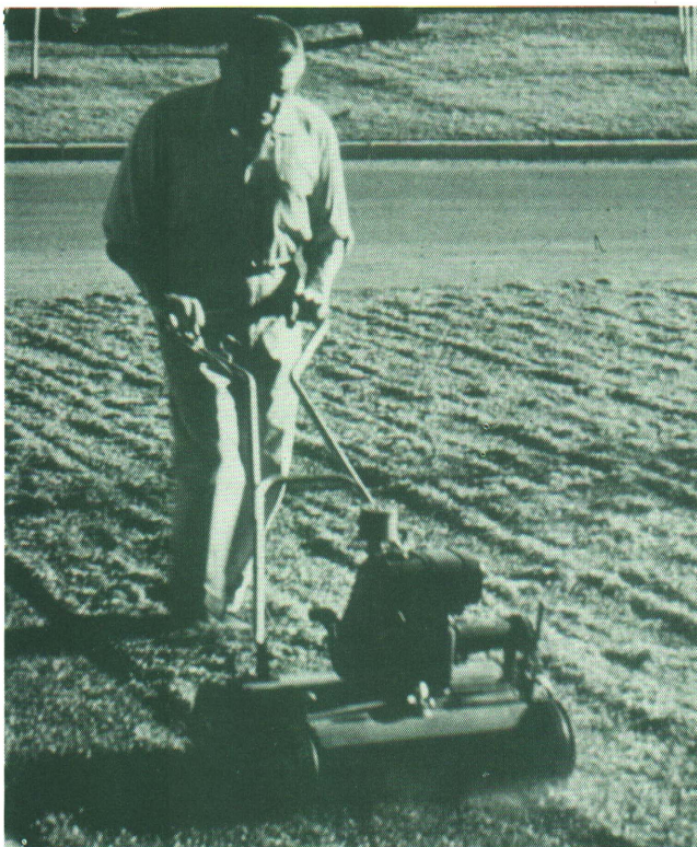
Thatch removal is best accomplished by using a de-thatching machine having vertical knives or tines. A de-thatching machine is more thorough than hand raking.
