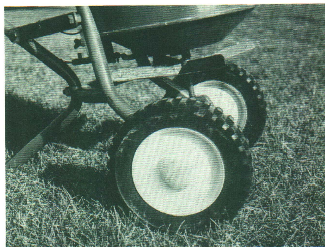
Centrifugal (broadcast) type fertilizer spreaders distribute materials rapidly with minimal overlapping.
