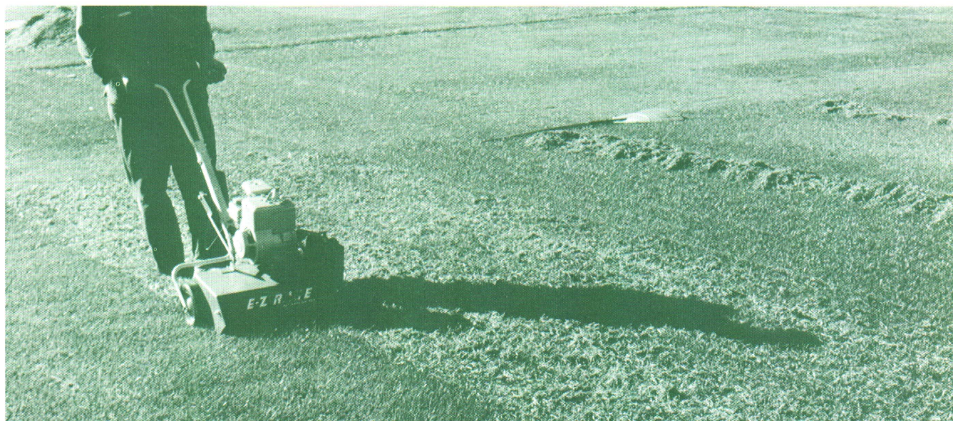
Thatch removal is best accomplished by using a de-thatching machine with vertical knives or tines. A de-thatching machine does a more thorough job than hand raking.
