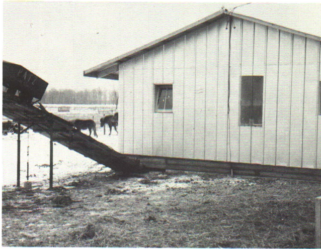
Figure 6—A gutter cleaner running through pens is a convenient system for moving manure.
