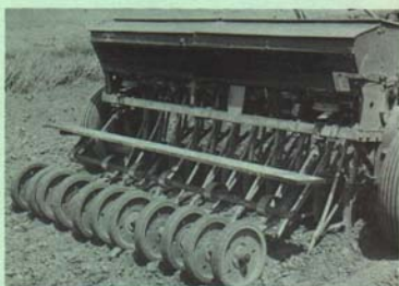
Figure 3. Seeding in early August should be with a band seeder followed by a cultipacker or press wheels to provide compaction for quick emergence and establishment of legume-grass mixture.
