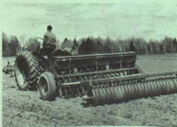
Figure 3. Seeding in early August should be with a band seeder followed by a cultipacker or press wheels to provide compaction for quick emergence and establishment of legume-grass mixture.
