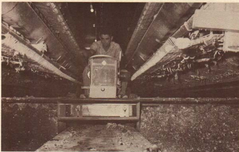
Fig. 13.—A small tractor with a wing-blade on each side can be used conveniently for removing droppings from below ceiling-suspended cages.
