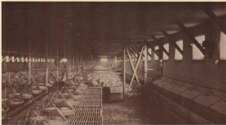
Fig. 8.—This floor management system provides a partial slatted floor, feeders on a track, and mechanical egg gathering equipment.
