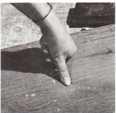
While sanding the soapy surface lightly, test for smoothness, using thumb or a piece of cardboard as a squeegee. When surface is uniformly smooth, stop sand-
