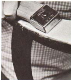
A cabinet scraper will remove some old finishes from flat surfaces.
