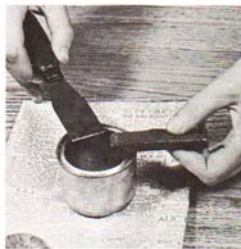
"Canned heat" can be used to melt a shellac stick for repairing deep scratches.
