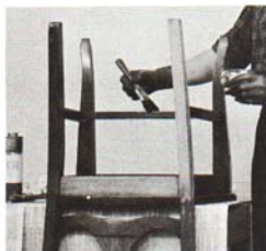
Start at the bottom first. Set chairs up-side down. Begin on underside of rungs.
