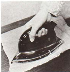
Pressure of warm iron on a damp cloth causes fibers in dented wood to swell. Wood should dry thoroughly.
