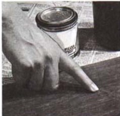
Filler is flattened and ready to wipe off if it rolls into a ball when you run your finger over the surface.
