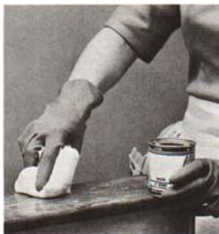
Apply paste wax with a cheese cloth pad. Spread evenly and smoothly. Buff with clean wool cloth.
