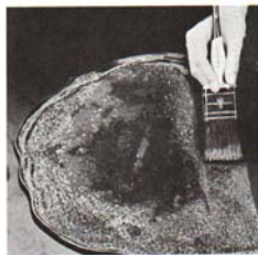
Stroke in one direction only as you apply remover. Don't brush it out.
