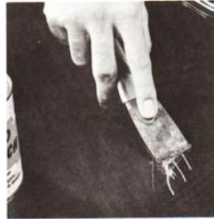
Tinted plastic wood applied with putty knife will repair deep chips and deep scratches.
