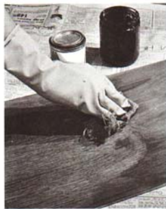
After the filler surface has flattened, wipe across the grain to force filler into pores.
