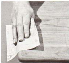
On curved surface, hold paper as shown above; press down with three fingers, work with the grain. Always sand with the grain. Press evenly throughout the stroke.
