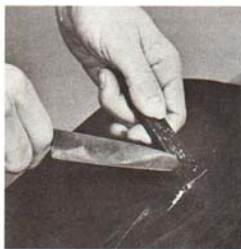
Warm a putty knife or spatula to apply the melted shellac to the wood surface.
