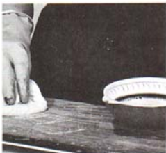
Sprinkle solution of water and hand dishwashing liquid on finished wood surface or apply with a cloth or sponge.
