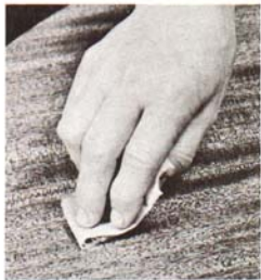
Fold paper into quarters and use without a block on turned areas, grooves, etc.
