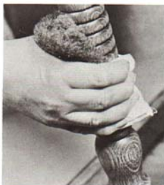
Steel wool is effective for removing finish from curved arms and legs.
