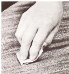
Fold paper into quarters and use without a block on turned areas, grooves, etc.
