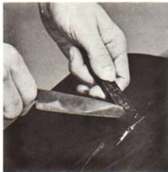
Warm a putty knife or spatula to apply the melted shellac to the wood surface.
