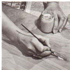
Enamel retouch will cover dark streaks on maple and other light colored woods.
