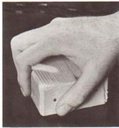
You can make your own by tacking abrasive paper to a wood block.
