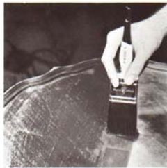
Apply stain with brush, cover thoroughly. Stain only one surface at a time such as leg, top, etc.
