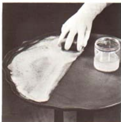
Mahogany table top, half of which is bleached. All woods do not bleach this well.
