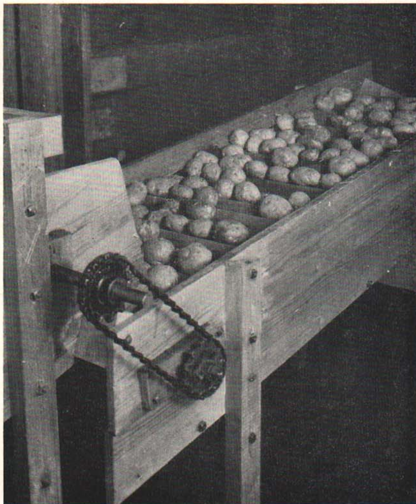
Fig. 7. Equip the grader with a roller-picking table to facilitate the removal of defective potatoes.
