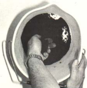
Mix the soil thoroughly—revolve the pail to ensure that a good mix is obtained.
