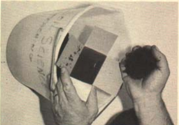
Place a pint of the soil in a clean container for transferring to the soil testing laboratory.
