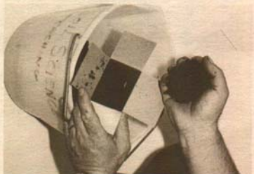
Place a pint of the soil in a clean container for transferring to the soil testing laboratory.
