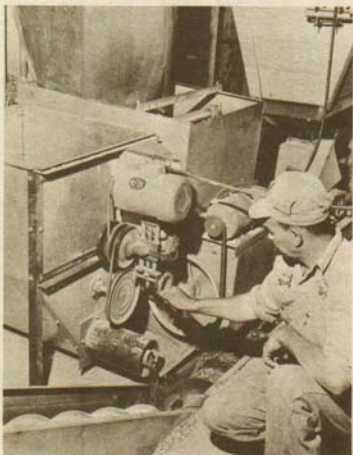
The hopper-bottom metal bin in foreground, coupled with the variable speed drive unit and changeable size augers in the bin, allow a wide range for metering grain, ground feed, and supplement. The rectangular metal bin (center) with a moving apron as a floor and the hoppers bin serve as meters or flow regulators for silage and cornage.
