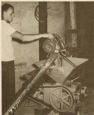
Roller used for cracking high moisture whole kernel corn. Auger with open screw section on end and variable speed drive acts as meter. High moisture corn unloads into small bins.
