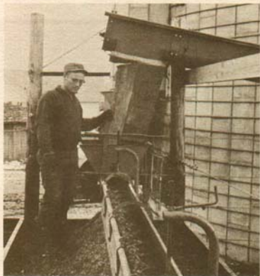
A trough-type auger conveyor feeds cornage into a metering hopper-bottom bin. Silage serves as the carrier for high moisture corn. Silage and cornage will be mixed by feeding auger.
