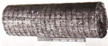
Fig. 34. This photograph illustrates the briquet made by the process shown in Figs. 27 and 31. The log produced measures 3¾ inches in diameter by 12 inches long and it weighs a little over 5 pounds. The ring structure of this log shows clearly in the photograph and is due to the manner in which the log is extruded through the single log tube. (Photo: Sumner Iron Works, a division of The Black Clawson Company).
