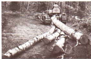
Fig. 2. Diesel tractor (48 drawbar horsepower) equipped with towing winch pulls logs from woods to landing. This operation would use three of these machines, each equipped with a skidding pan (not shown) to decrease skidding resistance and thus increase the number of logs hauled per trip. It is estimated that these three units will bring 40,000 board-feet of logs to the access road landings each 8-hour shift. (Photo: Caterpillar Tractor Co.)
