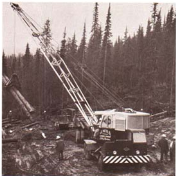
Fig. 5. Mobile log loader equipped with a 52-foot pipe boom and log grapple. The machine shown is considerably larger than the unit needed for this operation, but it illustrates the principle. In the proposed operation, 40,000 feet of logs must be loaded from the access road cold deck to sawmill-bound log trucks each 8-hour shift. The single operator not only controls the crane action but can also maneuver the truck. Use of a grapple eliminates the need for a log tong setter. (Photo: Baldwin-Lima-Hamilton Corp.)
