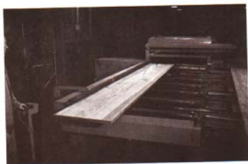
Fig. 18. Remotely-controlled, power-shift edger. Saw positions are indicated by special scales readily visible to operator. The edger delivers square-edged lumber to the grading chain. Edgings and sawdust are not wasted but are converted into fuel briquets for fireplace use. (Photo: The Ivory Pine Co.)
