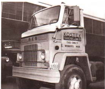
Fig. 7. A 220-horsepower cab-over tractor with 9,000-pound front axle and 22,000-pound rear axle. The cab-over design will permit maximum load lengths and still meet local regulations governing maximum loads. Three such tractors with matching trailers are needed to transport 40,000 board-feet of tree-length logs from woods to mill in an 8-hour shift. (Photo Reo Motors, Inc.)
