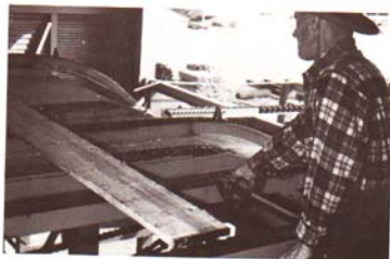
Fig. 22. Following the secondary manufacturing operations of surfacing and/or resawing, the lumber is sorted according to width, thickness, grade, etc. This view shows the sorter operator controlling the diversion of boards into a multideck sorter. The position of the slider bar operated by his right hand determines which level the board will seek. Each level of the sorter contains a particular grade or size of board. (Photo: The Ivory Pine Co.)
