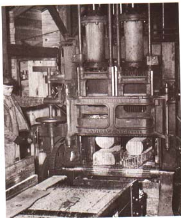
Fig. 17. Sash gang saw measuring 32 inches between styles or sash, with a stroke of 13 inches, depth of cut of 14 inches, and with 15½-inch maximum opening between feed rolls and press rolls. Note individual pressure cylinders actuating the split press rolls to permit feeding of multiple cants. By feeding cants in multiples, the gang-saw can maintain a production of 40,000 board-feet per 8-hour shift. (Photo: Wickes Brothers Division, The Wickes Corp.)
