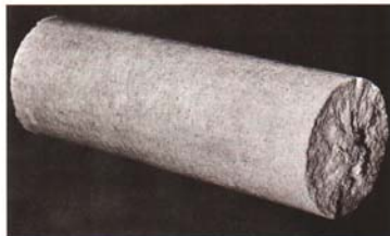
Fig. 33. This photograph shows the type of briquet made by the process illustrated in Figures 28 and 32. The log measures 4½-inches in diameter and weighs about 8 pounds. It burns with practically no smoke and leaves almost no ash. (Photo: Wood Briquettes, Inc.)
