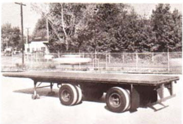
Fig. 8. Twenty-ton capacity trailer with 109-inch tandem to permit maximum loading and still meet local load limitations. Because of the necessity of hauling numerous short logs that develop along with the tree-length logs, a modified platform trailer may serve better than a conventional log trailer. Three such trailers, modified for carrying logs of mixed length, are required for the operation. (Photo: Trailmobile, Inc.)
