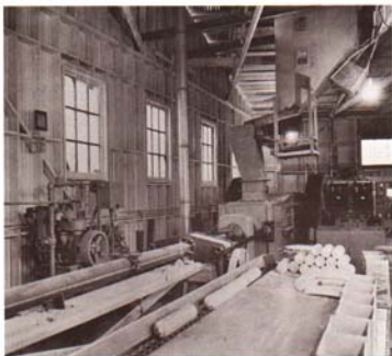
Fig. 31. Extrusion through this press is the final major step in the manufacture of fireplace-size log briquets from wood waste. Dry refuse (of controlled particle size) is admitted from the overhead storage hopper. The log tube extends to the left. Capacity of this machine ranges up to 2 tons per hour. See Item 37 in Fig. 27 for the location of this equipment in the manufacturing process. (Photo: Sumner Iron Works, a division of The Black Clawson Company).
