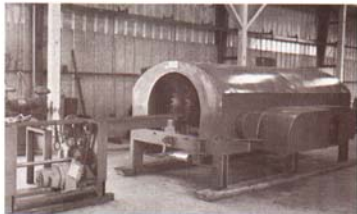
Fig. 13. Infed end of a multiple-saw pole (or "scrag") mill. The saws can be spaced by remote control to cant each log with a minimum thickness slab. The feed works is provided with a log turning device which positions the log for maximum yield. The feed chain is continuous through the machine, and logs travel straight through in an uninterrupted fashion. (However, if an occasional log requires it, the feed chain can be reversed and the cant brought back to the infed end; then, the saws can be re-spaced and side cuts taken on a second pass.) The machine for this operation should carry only one pair of saws. (Photo: Keystone Machine Works)
