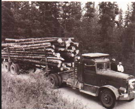
Fig. 6. This photograph (from an enterprise in eastern Washington) shows a 40-ton maximum capacity truck with a load of lodgepole pine logs in the same diameter class as the hardwoods involved in the operation under consideration. Because of local load limitations, more trucks (having a load limit of only 20 tons each) must be used in this operation. (Photo: Biles-Coleman Lumber Co., Inc.)
