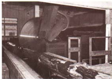
Fig. 9. Circular, 48-inch diameter swing cutoff saw with air fed cylinder. Log dogging jaws which will accommodate themselves to burly or uneven logs are visible to the left of the saw line. Here logs are bucked into exact lengths ranging from 8 to 12 feet to produce a multiple of the desired pallet board length. This equipment is located at D in Fig. 10. (Photo Sumner Iron Works, a division of The Black Clawson Company).
