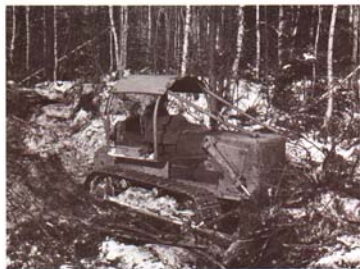
Fig. 3. Diesel tractor (75 drawbar horsepower) equipped with bulldozer and towing winch builds a winter haul road on a logging job. One such machine would be needed to build access roads for the three 20-ton capacity logging trucks. (Photo: Caterpillar Tractor Co.)
