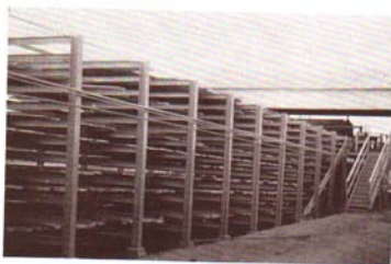
Fig. 23. View of a multideck lumber sorter looking from the sawmill in the direction of lumber movement and toward the lumber stacking station at the far end. Each level of lumber represents a separate sort. As each level fills with lumber, it is emptied onto powered chains that convey the entire sheet of stored boards to a mechanical stacker. (Photo: The Ivory Pine Co.)
