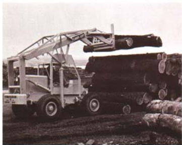
Fig. 11. All movement of logs in the mill area (from log sorter to log storage and from log storage to sawmill deck) is handled by this versatile four-wheel drive forklift. It is estimated that one operator with such a machine can keep the mill supplied with 40,000 board-feet of logs per shift. (Photo: Pettibone Mulliken Corp.)
