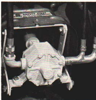
Fig. 11. — Sliding vane impeller pump.
