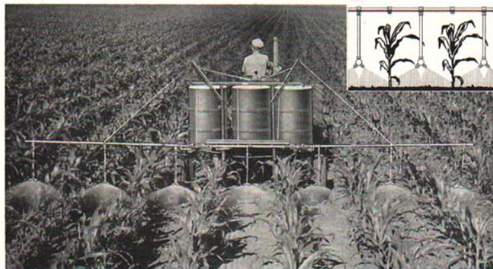
Fig. 16. — Drop pipes for corn herbicide application.
