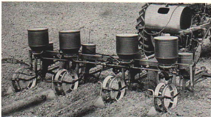
Fig. 24. — Corn planter with herbicide applicator.
