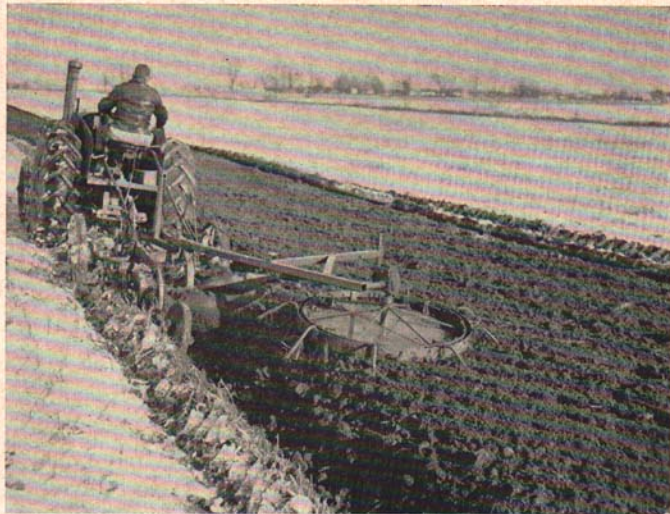
Fig. 8. This circular tiller revolves as it is pulled behind the plow. You can add weight to the wheel for more firming.
