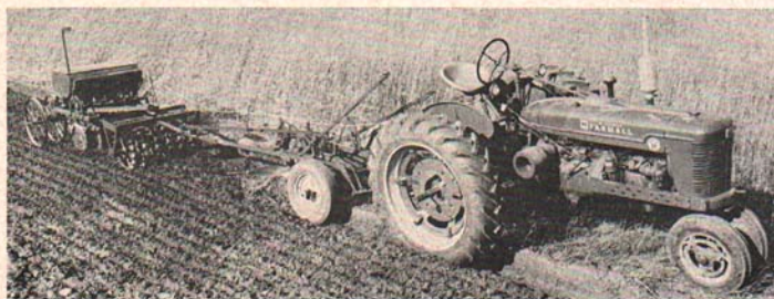
Fig. 2. The plow packer and press drill combination has been a very good method for planting oats and legumes. Note the good soil condition following the drill. Seeding is through five straight disk openers. A packer wheel follows each opener. Soil is pressed on the seed to aid in quick germination.
