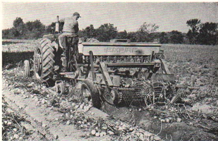
Fig. 4. On potatoes dug early enough in the fall, a rye cover crop may be planted at the same time, by attaching a seeder box to the digger.
