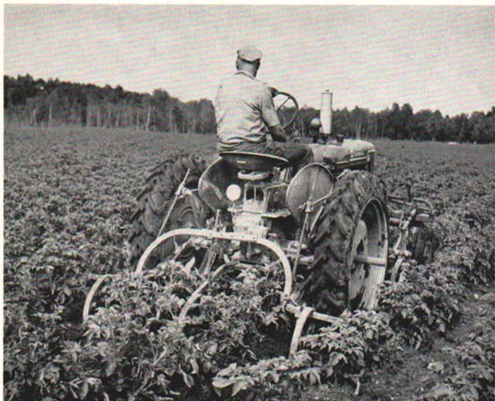
Fig. 6. This picture illustrates cultivation late in the growing season with the teeth of the cultivator operating mainly from the middle of the row.
