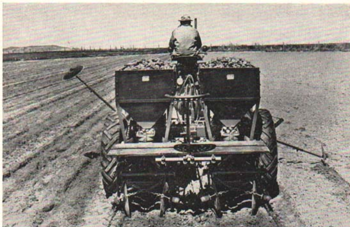
Fig. 5. This picture illustrates the proper adjustment of the covering discs on the planter to avoid covering the seed with too thick a layer of soil.
