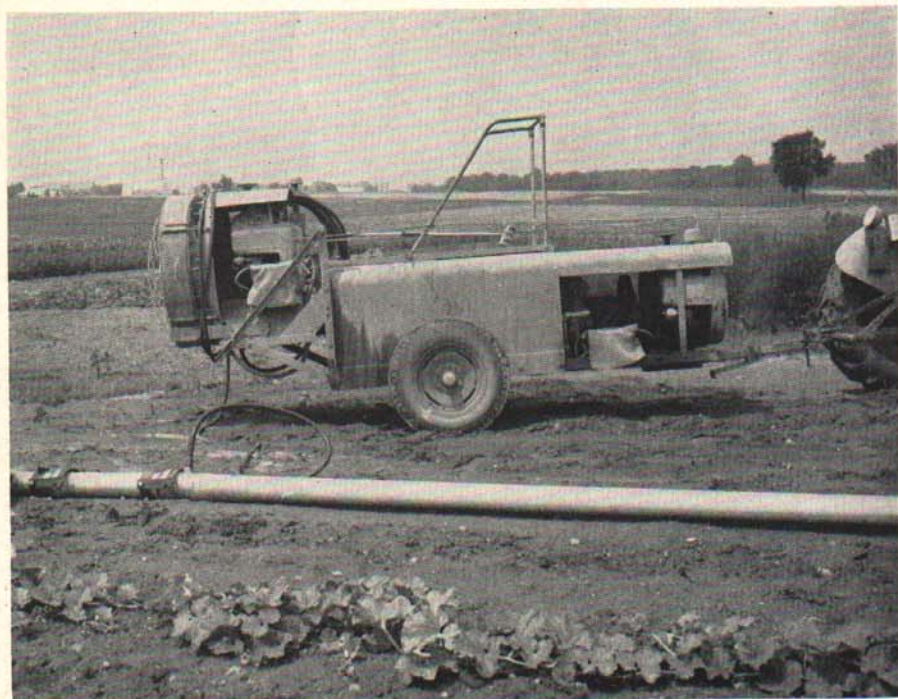
Fig. 3. Using a spray rig to pump a fertilizer solution into an irrigation pipeline.
