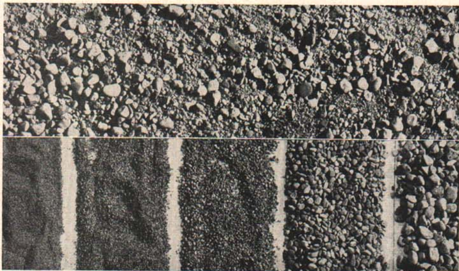
Fig. 1. Well-graded sand, before and after being separated into various sizes. Particles vary from fine to those that will just pass through a No. 4 sieve.
