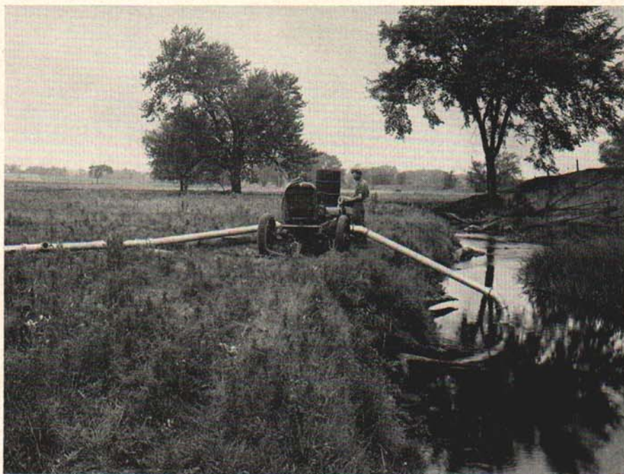
Fig. 2. For an efficient operation, irrigators depending on streams for their water supply must base plans on the flow "during the driest time of the driest years." The mobile unit pictured can pump 30,000 gallons an hour.
