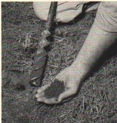
Fig. 3. Taking a soil sample with a soil auger.
