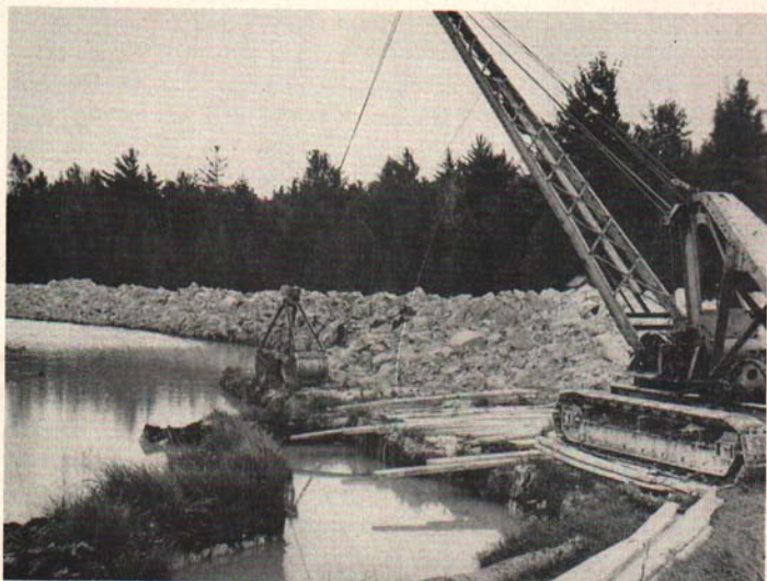
Fig. 4. Michigan has extensive deposits of marl, a good liming material if always tested first for "purity," so that its rate of application can be properly calculated. Many of the marl beds are of the size and quality to warrant commercial operation on the scale pictured here.
