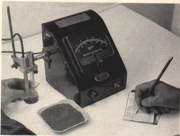
Fig. 1. A "pH meter" is employed in determining the soil reaction, or acidity, used as a basis for lime recommendations. An adaptation for soil-testing purposes of the standard "potentiometer"—long in use for the scientific measurement or comparison of electrical potentials—the meter is calibrated so that its dial reads directly in pH values. (Greatly simplified, the working principle is this: In each case, the degree to which a soil is acid or alkaline has a measurable effect upon certain basic relationships of electrical energy. Those relationships are established when the electrodes [at left] are thrust into a sample of soil mixed with water. The instrument then measures the effect with great accuracy, and indicates the result in terms of the pH scale.)
