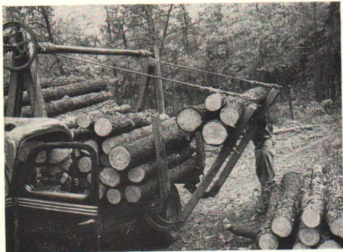
A self-powered truck loader for heavy box-bolts. Arms of the loader rest on the ground; rope hoists are unbooked, when bolts are rolled onto the arms. Brackets (not visible) keep bolts in place when the arms are hoisted.
