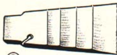
D. Creased bucking wedge. Brightly colored cord tied through hole makes it easier to locate and pick up after use.
