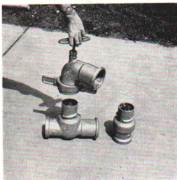
Fig. 8. Pipe couplings used in supplemental irrigation. (A) No latch lock. (B) Single latch lock. (C) Double latch lock. (D) Tractor-tow latch lock.
