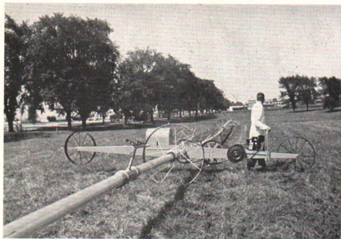
Fig. 11. A side roll irrigation lateral power moved by a small engine.
