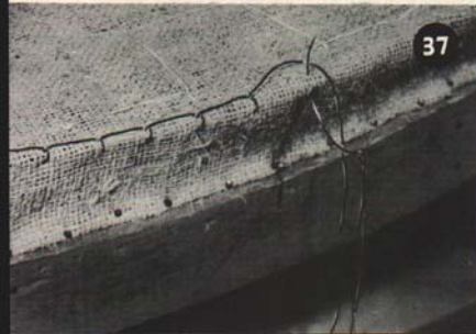
FIGURE 37. With mattress twine and a curved needle sew the burlap to the front wire edge. This is in preparation for making the heavy front roll.
