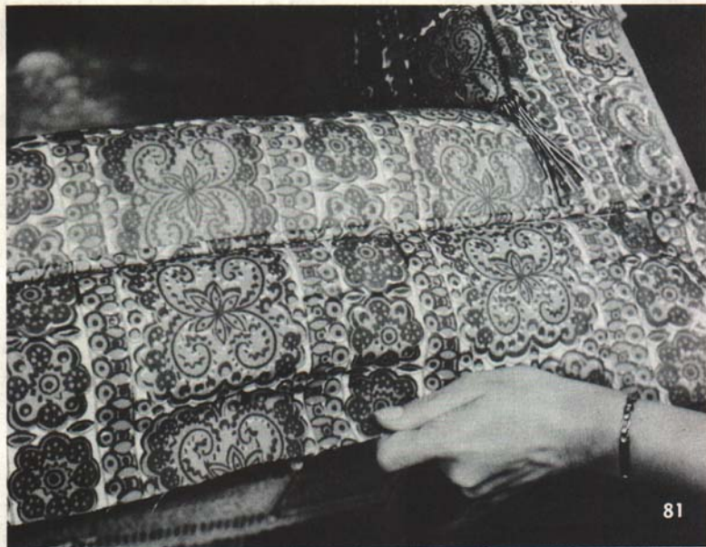
FIGURE 81. Pull the fabric down until it is very taut. Tack it underneath the chair, working from the center to the sides of the chair. Slash the fabric, if necessary, at the corner of each leg before completing your tacking.
