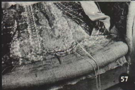
FIGURE 57. Pin and stitch the seam securely to the burlap base with a mattress twine and curved needle.
