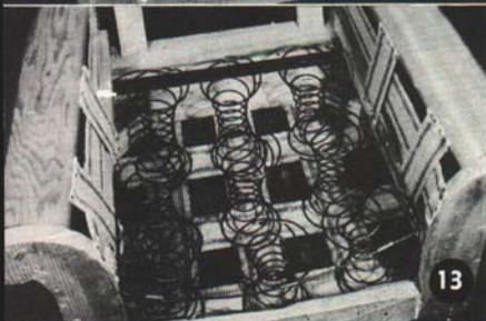
FIGURE 12. Place the spring right side up on the interlaced sections of the webbing.
